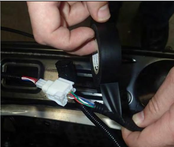
13. Apply electrical tape to insulate exposed areas of loom and hold convoluted tube as shown.
