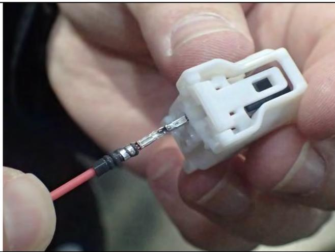
11. When rehousing crimped terminals into the new female plug, make sure that the orientation of the terminal is such that the crimp bucket is facing up towards the clip as shown.
