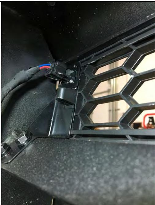
15. Plug the open end of the supplied loom into the back of the camera and check for operation, zip tie loom to ensure movement is limited and it is well clear of any moving parts. Check there is no exposed wires at the camera end and they are protected by the conduit, use electrical tape to fix the conduit in position.
