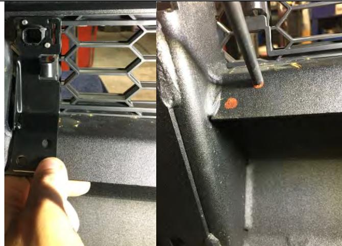
4. Place bracket in position and mark with a pen or transfer punch.
