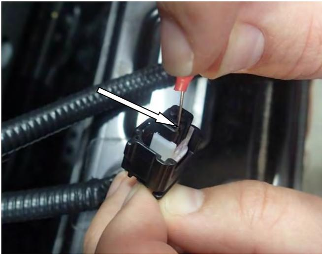
8. Using a sharp point, push down front of terminal while gently pulling wire out from the back of the plug.
