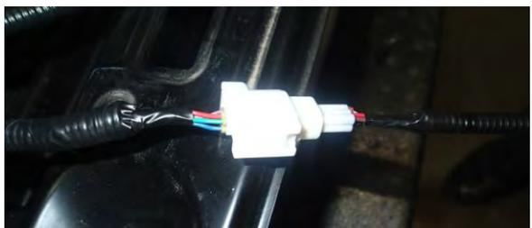
14. Plug the supplied camera loom into the connector (now part of vehicle loom) and route down under the grill so it can be plugged into the camera.
